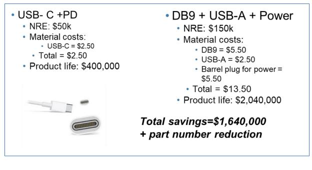
Figure 7: Cost comparison of USB–C + PD
